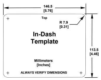
In-dash mounting template for FishEasy 250DS, showing dimensions. The preceding figure is *not* printed to scale. A scaled template is available for free download from our web site, www.eaglesonar.com.
